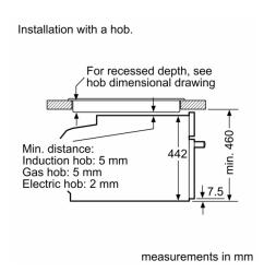
If the compact appliance will be installed underneath a hob, the following worktop thicknesses (including substructure if necessary) must be taken into account.
